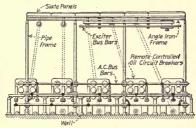
Fig. 229.—Plan view of the mechanical remote-control switchboard.
